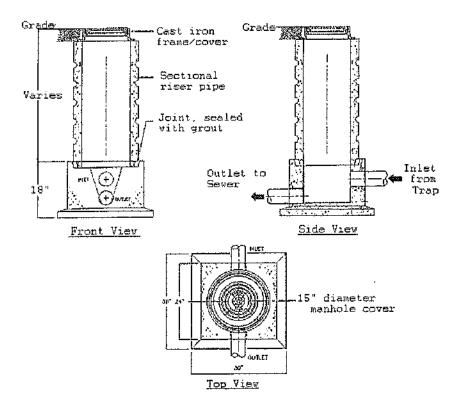
2. Sampling wells will have a minimum 15" diameter access with ring and lid and a minimum 4" drop from inlet to outlet piping through the sampling well.
